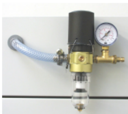
Figure 13: Compressed air connection with condensate separator
