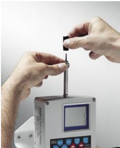
3) Lift the protection cap without touching the sensor
