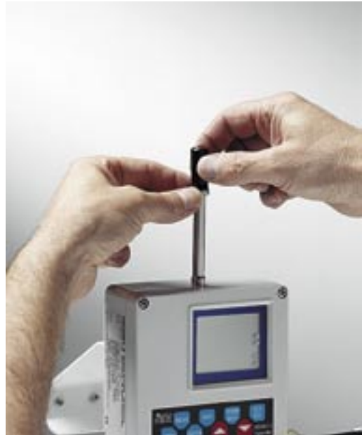
2) Keep the ring nut fix, then screw the protection
