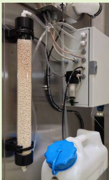
\text{CO}_2 scrubber and integrated water tank
