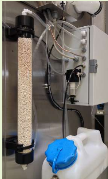
CO 2 scrubber and integrated water tank
